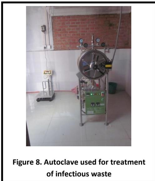
**Figure 8. Autoclave used for treatment of infectious waste**
